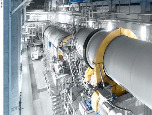
Thanks to cost-efficient and environment-friendly technology, the TwinDrum pulper system offers excellent ink removal and gentle breaking down of fibres in the stock preparation process of the paper production.
