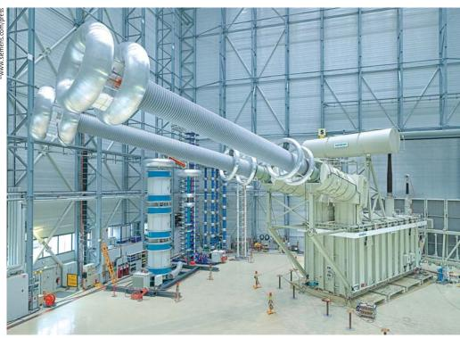
For the world's largest high-voltage direct-current (HVDC) transmission line in China Siemens worked in tandem with Chinese partner companies to develop HVDC transformers which are among the most powerful in the world with a capacity of 587 megavolt-amperes.
