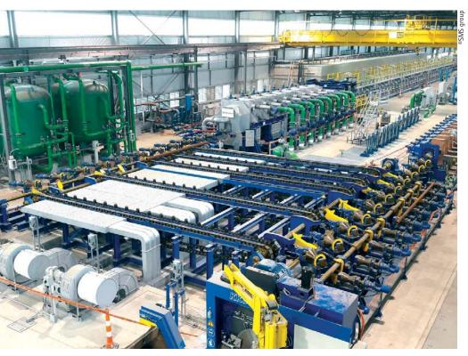
The new state-of-the-art heat-treatment line supplied by SMS group to TimkenSteel has the capacity to produce 50,000 tonnes of bars and tubes for the automotive, industrial and oil and gas industries.
