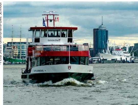
The latest harbour ferries built by the Hamburg-based shipbuilder Pella Sietas boast a hybrid propulsion system and further technological innovations that reduce their environmental impact.
