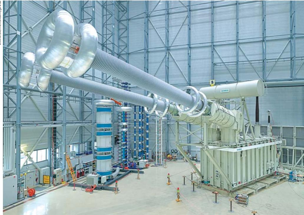
For the world's largest high-voltage direct-current (HVDC) transmission line in China Siemens worked in tandem with Chinese partner companies to develop HVDC transformers which are among the most powerful in the world with a capacity of 587 megavolt-ampères.
