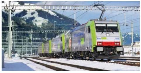
The TRAXX F140 multi-system (MS) / Re 486 locomotive is used by the Swiss firm BLS Cargo to provide freight services between Germany and Switzerland.
