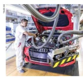
Combination fluid filling during production of the Audi A3 at the company's Ingolstadt site.
