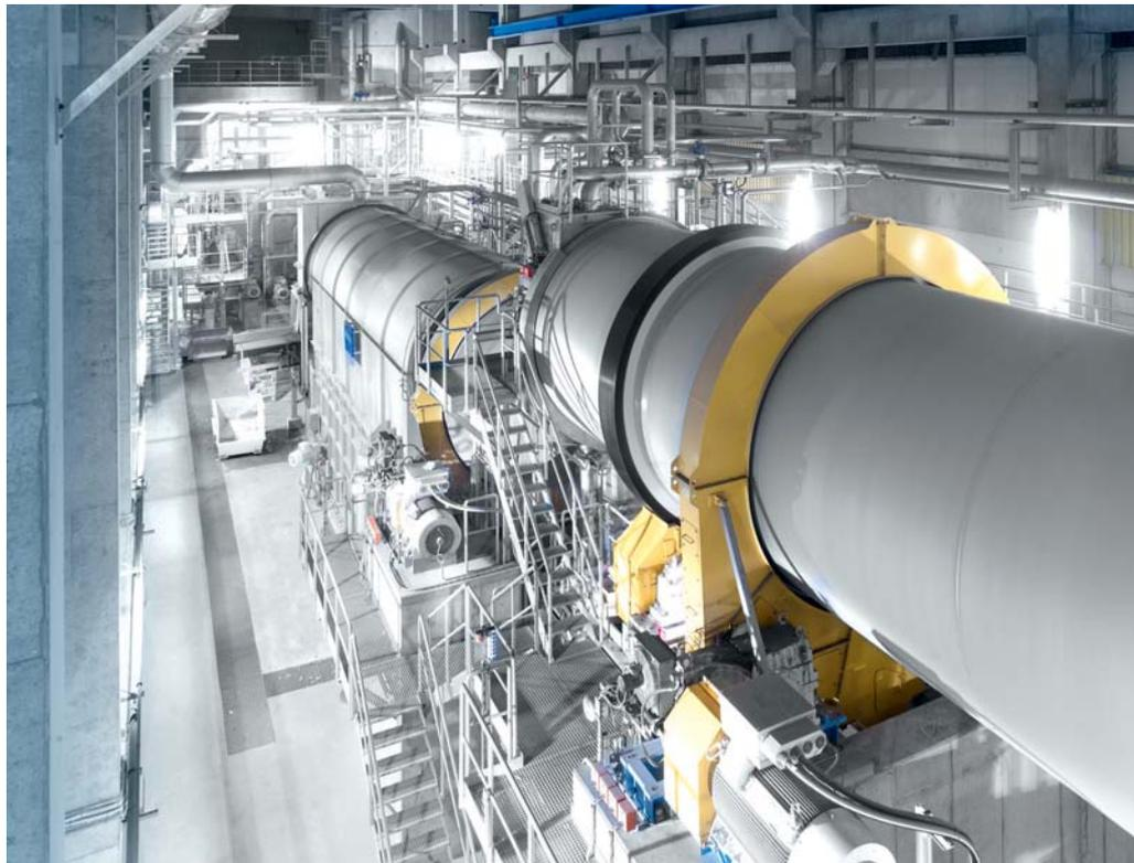
Thanks to cost-efficient and environment-friendly technology, the TwinDrum pulper system offers excellent ink removal and gentle breaking down of fibres in the stock preparation process of the paper production.
