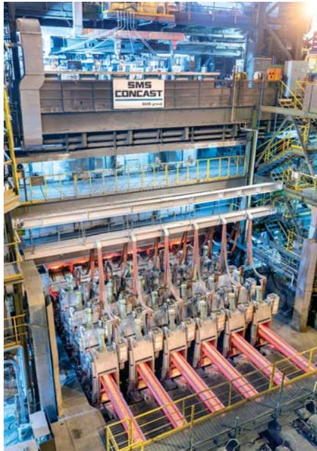
The revamped SMS Concast continuous casting machine in full operation at Hyundai Pohang, South Korea.
