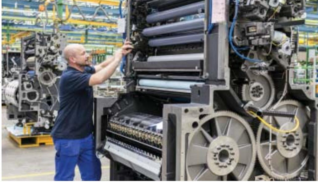
Highly skilled engineers, technicians and fitters are key to the success of the German engineering industry – Assembly of a Speedmaster XL 106 printing machine.
