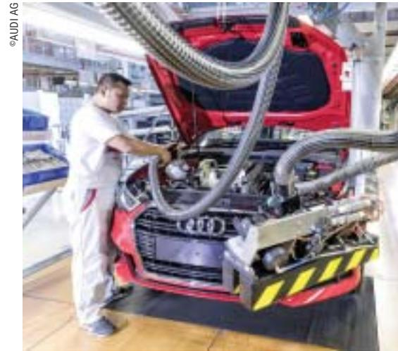
Combination fluid filling during production of the Audi A3 at the company's Ingolstadt site.
